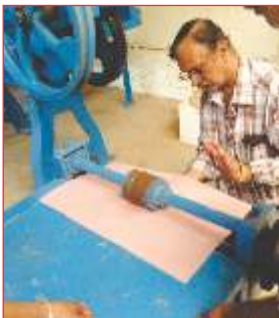
Mr. Ravikumar Checking The Creasing Machine
